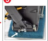
After the handle is clipped on, tighten the wingnut.
