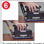
To remove the handle, loosen the wingnut, hold the handle upright and turn the handle to the side to release it.
