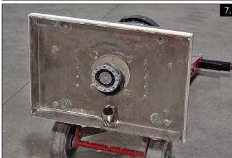
8. Using a 7 /16" socket, remove the cap bolt from the motor shaft.
