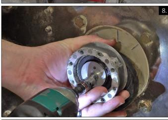
9. Remove the crush washer from the bearing.
