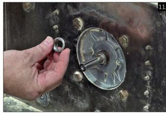
12. Replace the old spacer with the new spacer included in the eccentric assembly repair kit. Apply silicone on top & bottom of spacer. Do not reuse old motor shaft spacer.
