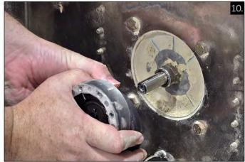
11. Remove the motor shaft spacer.
