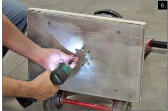
7. Remove the aluminum plate. Clean debris or build-up if needed.
