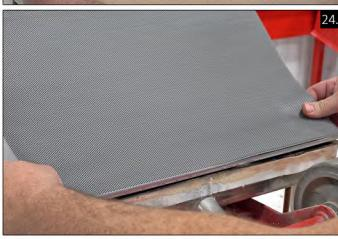
25. Smooth evenly, while slowly pulling the liner until completely removed and press firmly around all areas of the grip face.
