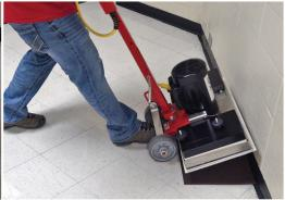
Place the pad against the wall, then tilt the machine back and place it on the pad.
