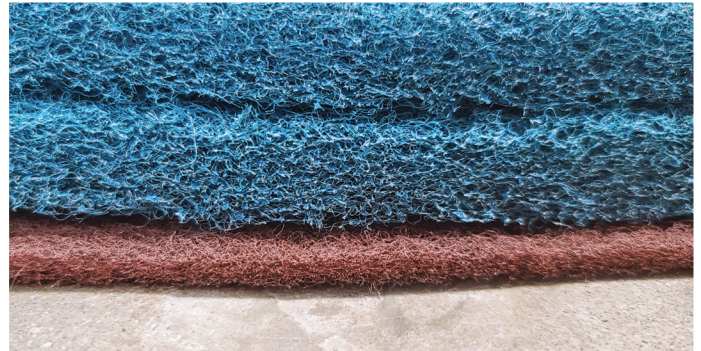
Stacking driver pads for uneven floor surface.
