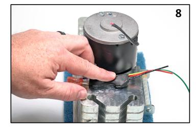
Set the new wiring harness in the silicon. Allow 2-4 hours for the silicon to completely dry.
