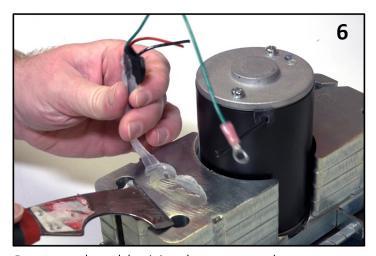
Remove the old wiring harness and any remaining silicon.
