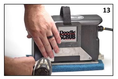
Lower the cover onto the Doodle Scrub® base. Align the carry strap, and install the 4 new cover screws.
