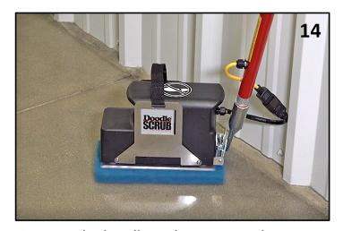
Connect the handle and power supply, and test the Doodle Scrub® on a driver pad.
