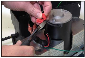
Cut both sets of black and red wires leading from the red wire connectors. Disconnect the black and white wires leading from the cover.
