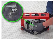
5. Tighten down the metal plate with the wing nut.
