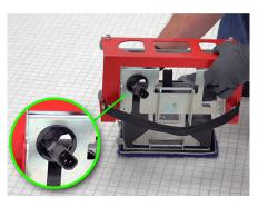
2. Lower the Skate down onto the Doodle Scrub® while feeding the power cord through the hole.
