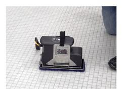
1. Disconnect the power connector and remove the handle.
