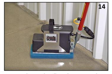
Connect the new handle and power supply, and test the Doodle Scrub® on a driver pad.
