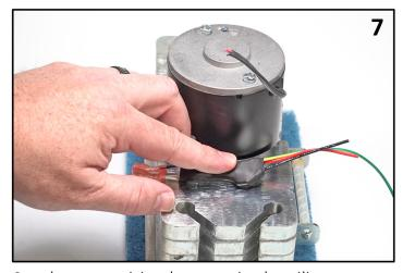
Set the new wiring harness in the silicon. Allow 2-4 hours for the silicon to completely dry.
