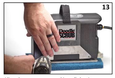
Align the carry strap, and install the 4 new cover screws.
