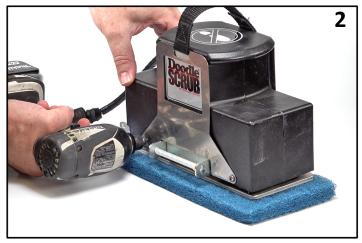
Use a Torx 20 to remove the 4 base screws. Remove the carry strap.
