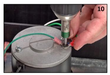
Connect both green ground wires to the motor using the new motor ground screw.
