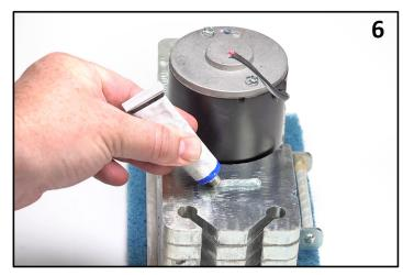
Apply a bead of silicon to the machine base.
