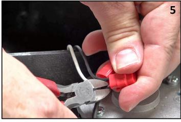
Cut both sets of black and red wires leading from the red wire connectors.
