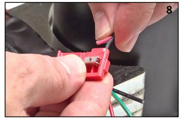
Insert the red wire from the motor and the red wire from the harness into the connector.
