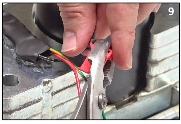
Clamp down using pliers. Repeat steps 8 and 9 with the black wire from the motor and the black wire from the harness.
