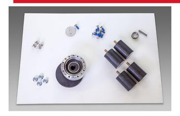
This kit contains everything needed to replace the eccentric assembly for the EBG-18 PIVOT. When replacing, Square Scrub recommends installing new isolators as well. Included are: 4 isolators, isolator bolts, motor shaft spacer, motor shaft cap bolt, bearing bolts, eccentric assembly, crush washer, eccentric assembly key, grip face, anti-seize, & 100% silicone. Only compatible with machine serial numbers beginning with 18P.
