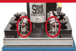
The 1/2" isolators connect the machine handle to the base, and help to reduce nearly all felt vibration. The 1/2" Isolator Kit includes: 10 1/2" handle Isolators & 10 isolator nuts.
