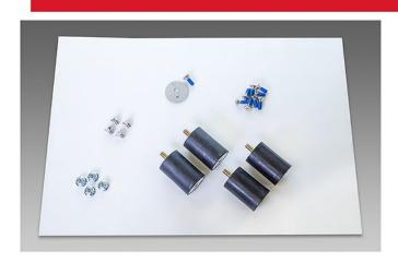
The Isolator Repair Kit has been created to make this standard maintenance process easier. Kit include: grip face, 4 isolators, isolator nuts & bolts, motor shaft spacer, motor bolt, bearing bolts, motor washer, 100% silicone and thread lock. Only compatible with machine serial numbers beginning with 20P.
