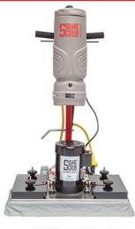
A standard EBG-28 PIVOT Floor Preparation Machine with the HEPA Dry Vac installed. For additional information on the EBG-28 PIVOT, see page 4. For additional information on the HEPA Dry Vac Kit, see page 4.
