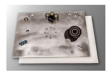
This kit contains everything needed to replace the eccentric assembly for the EBG-20/C. When replacing, Square Scrub recommends installing new isolators as well. Included are: aluminum driver plate, 4 isolators, isolator bolts, motor shaft spacer, motor shaft cap bolt, bearing bolts, eccentric assembly, crush washer, eccentric assembly key, grip face, anti-seize, & 100% silicone.
