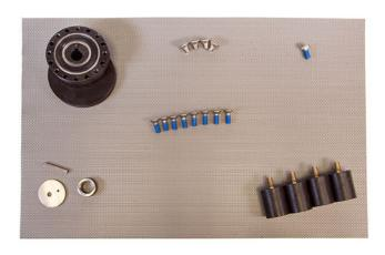
This kit contains everything needed to replace the eccentric assembly for the EBG-20/C. When replacing, Square Scrub recommends installing new isolators as well. Included are: 4 isolators, isolator bolts, motor shaft spacer, motor shaft cap bolt, bearing bolts, eccentric assembly, crush washer, eccentric assembly key, grip face. Not shown: anti-seize, & 100% silicone.
