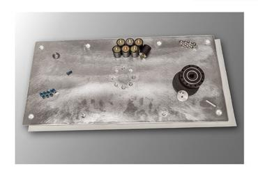
This kit contains everything needed to replace the eccentric assembly for the EBG-28. When replacing, Square Scrub recommends installing new isolators as well. Included are: aluminum driver plate, 8 isolators, isolator bolts, motor shaft spacer, motor shaft cap bolt, bearing bolts, eccentric assembly, crush washer, eccentric assembly key, grip face, anti-seize, & 100% silicone.
