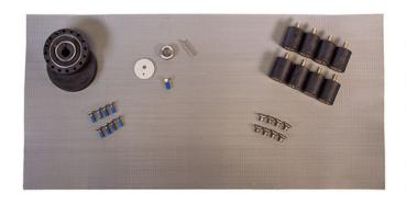
This kit contains everything needed to replace the eccentric assembly for the EBG-28. When replacing, Square Scrub recommends installing new isolators as well. Included are: 8 isolators, isolator bolts, motor shaft spacer, motor shaft cap bolt, bearing bolts, eccentric assembly, crush washer, eccentric assembly key, grip face. Not shown: anti-seize, & 100% silicone.
