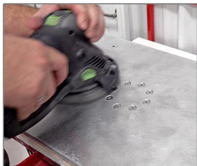
4. Abrade the plate using an orbital sander with 80 grit sandpaper to remove a very thin layer of aluminum evenly.
