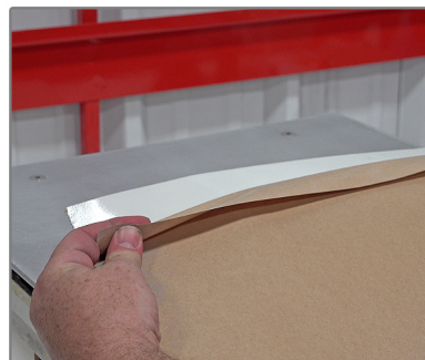
6. Remove back liner of the new grip face 2" from the long edge.
