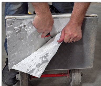
1. Remove old grip face from the plate.
